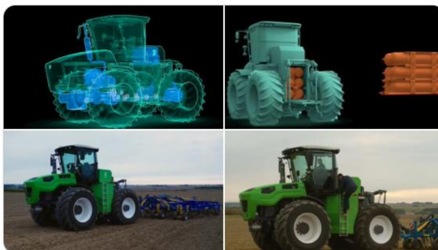
Source: Auga, picture of M1 tractor: 12 hours runtime, 500 equivalent hp, biomethane gas – electric drive system, changeable biomethane gas cartridges (2-3 min to change)
